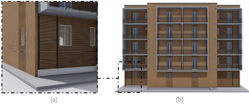
Figure 7.9. (a) Architectural integration of expansion joints on the building façade and (b) north front of the case study at post-intervention state.
