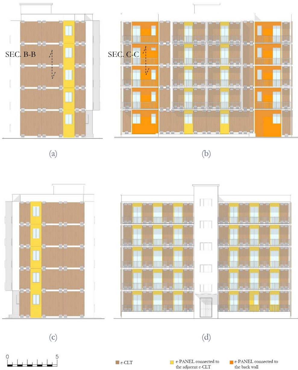
Figure 7.4. Application of e-CLTs and e-PANELs on the: (a) east front, (b) north front, (c) west front, (d) south front of the case study.
